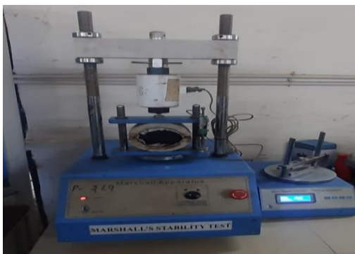
Fig. 1: Marshall’s testing apparatus
